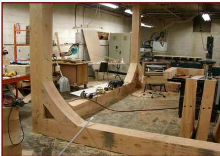
Mortised Cedar Millwork, pre-assembled in-house to Architect's Specifications
